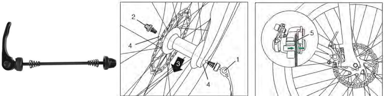
4.3 Ensure that the installation direction of the front wheels is correct. Make sure fork hanger hold onto wheel axle, and make sure the disc put into middle of brake.
