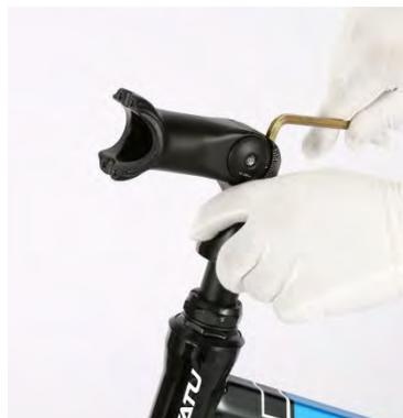
3.2 Using the wrench from tool kit to loosen the four screws and put the stem into the bike in balance and you can adjust the handlebar in a property angel and position.
