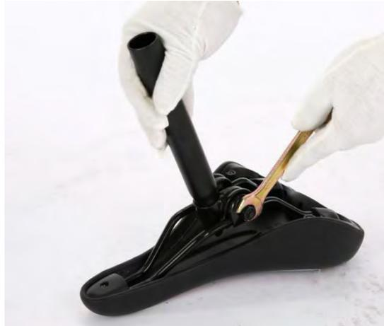
7.2 Insert seat post into post receiver, set right its position and adjust height to fit your riding habit. Then, Tighten seat by clamp.
