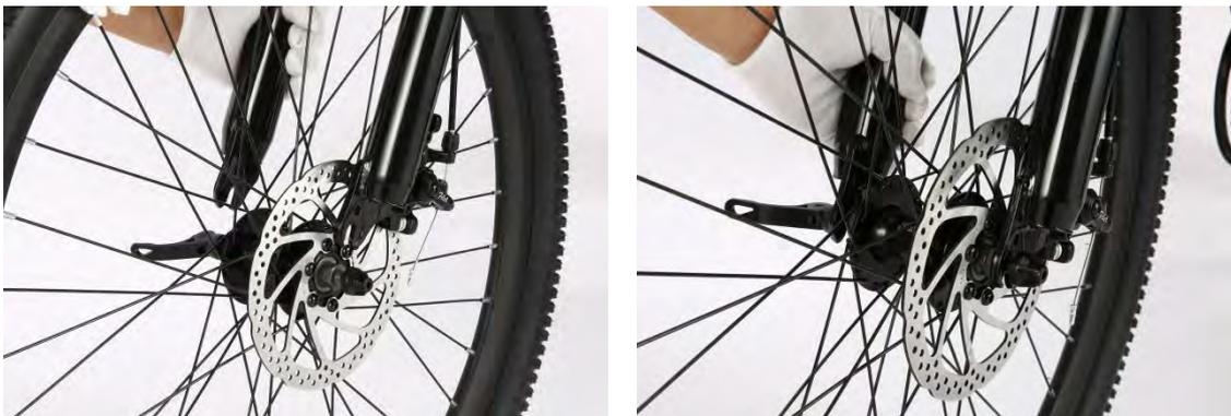
4.4 Insert quick-release axle into spring and tighten screw(Quick release nut to be at the same end as the brake).
